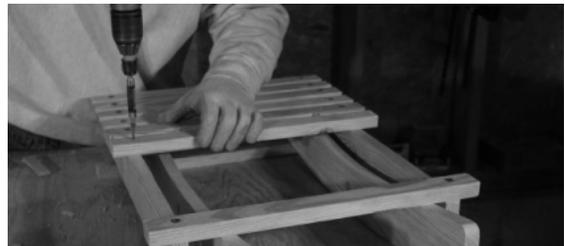
**03** Cut all dowels to length, turn the stretchers/one slat assembly over and slip one table dowel (E) through the outer legs and stretchers at the end opposite the attached slat. Make sure the dowel ends are flush with the outside face of the stretchers and attach with glue and 6d finish nail (drill a  $\frac{1}{16}$ " pilot hole through the edge of the stretcher and into the dowel, then drive the nail below edge surface of the stretcher with a nail set).
