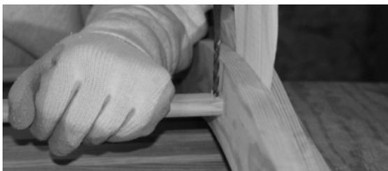
**TIP:** This is one of those projects that may be more easily sanded and finished without all the pieces connected. If you choose this method, do an initial assembly without glue to make sure all pilot holes and edges line up and appear to your liking. Then disassemble, sand smooth, and reassemble with glue and screws.
