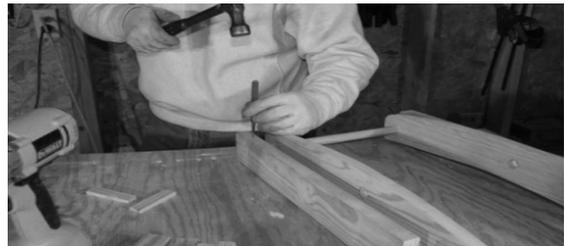
**02** Rip your remaining 1 x 6 stock to  $1\frac{3}{4}$ " wide and cut 11 slats (C) 16  $\frac{1}{2}$ " long. Place one slat on top of the stretchers (B) at the end with the slot (not the hole) and attach with glue and screws. Leave  $\frac{1}{2}$ " overhang on the front edge and 1" on either end.
